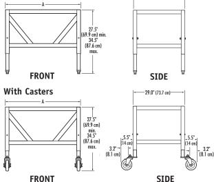
*Telescoping Base Stands provide support for XPert Balance Enclosures.*\*
