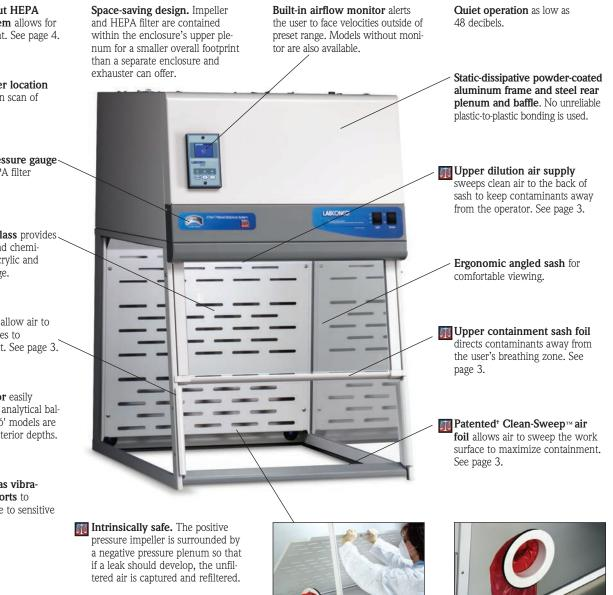
Patented<sup>†</sup> rear baffle with zones of perforations promotes horizontal laminar airflow. See page 4. The baffle pivots down for cleaning. Optiona waste c waste in and 6' m chute. C
