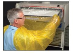
can remove a contaminated filter without exposing the filter or contaminated plenum to personnel or the environment. On XPert Filtered Balance Systems and Stations, the filter is accessible by remov-
