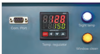
Electronic over temperature shutdown system.
