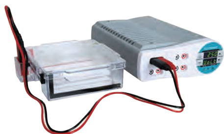
Connection to Power Supply
