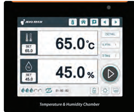
Color touch display controller (5.6 inches)
