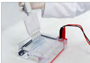
Comb spacing fitting to Multichannel pipettes (31, 16 well Comb).
