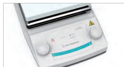
Top plate overheating indicator light.
