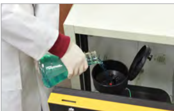
Wide inlet of waste liquid funnel.
