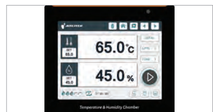
Controller for temperature and humidity control. (TH3-model)
