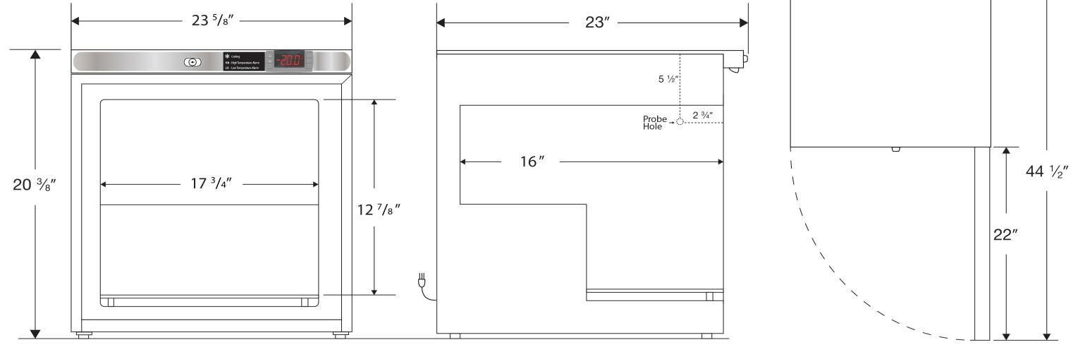
Note: This unit must have 4" clearance on sides and back for adequate ventilation
