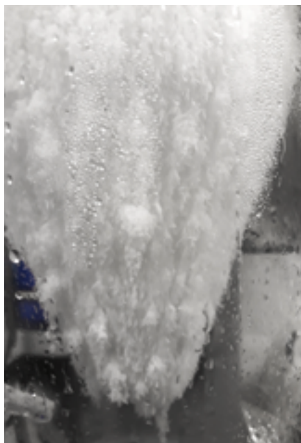
Fig. 2: Ice crystals from humidity form in the dry ice chiller between applications
