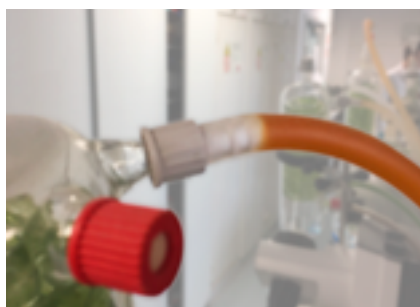
Fig. 3: Algae formation in the cooling coils and cooling water hoses
