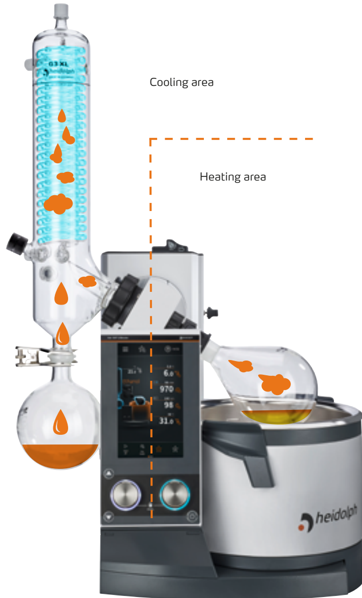
Fig. 1: Evaporation process on rotary evaporator
