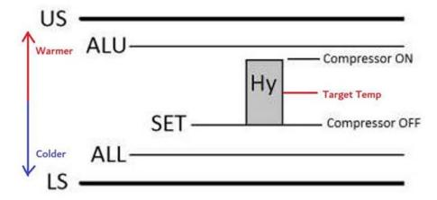
During the normal operation, the refrigerators (or freezers) compressor would turn on and off, to maintain the cold temperature in the storage chamber.
