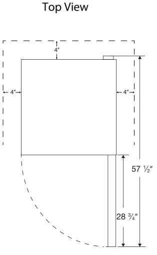
NOTE: Ventilation Requirements – Minimum 4" clearance on sides and back
