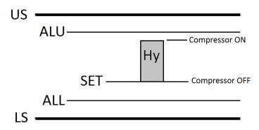
During the normal operation, the refrigerator's (or freezer's) compressor would turn on and off, to maintain the cold temperature in the storage chamber.
