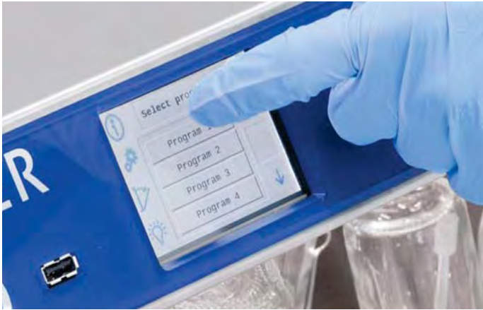
The Prolux PLC Controller includes a touchscreen interface with a common icon directory that permits scrolling access to primary screens from the same menu. A set of sub-menu screens display additional icon directories specific to the screen functions.
