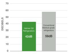
Every increase of 10dB on the scale is equivalent to a 10-fold increase in sound intensity. U/C refrigerator example shown.
