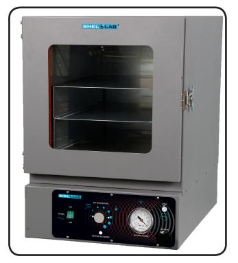
SHEL LAB vacuum ovens provide exceptional capabilities for fast and gentle drying of heat sensitive materials. They prevent residue accumulation on products and also allow safe drying of flammable solvents.
