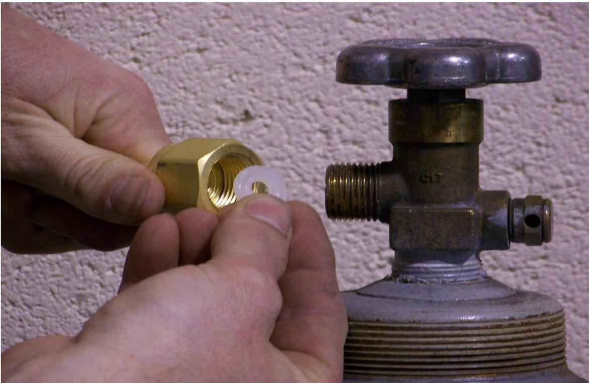
6. Securely tighten each line with wrench. You may now open the tanks and adjust your regulator.
