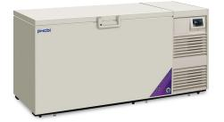
The patented TwinGuard -86°C chest freezer is powered by a unique concept of two independent auto-cascade cooling circuits that work together, both independently and concurrently, to provide continuity in stored product protection over a range of real world conditions.
