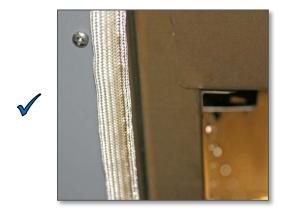
Figure 9: Chamber Gasket Aligned
