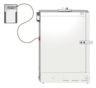
**2.** Position the sensor probes in the chamber.
