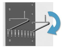
Figure 5: Install Clips
