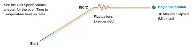
**Heat Up and Stabilization Phases**
