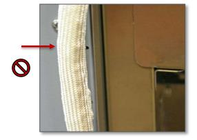
Figure 8: Chamber Gasket Misaligned
