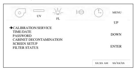
Entry into the Calibration/Service functions requires a service password for entry. After pressing Calibration/Service menu item, a password screen will appear. The default password is "9876". Once the service password is entered the Calibration/Service menu will appear.
