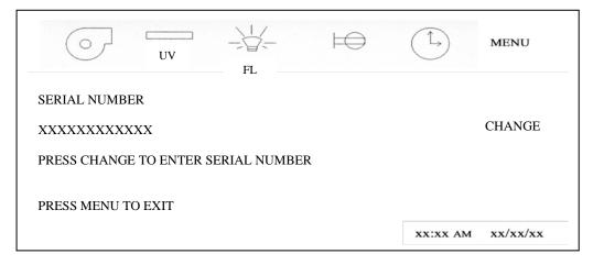
• Once CHANGE is pressed, a display screen very similar to the password display screen will appear for entry of the serial number. After entry of the serial number press ENTER to save the serial number.
