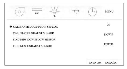
Step 2: Press CALIBRATE DOWNFLOW SENSOR to access individual calibration screen. Press BLOWER switch to on. Allow blower to run for one minute or until downflow readings are steady.
