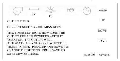
UV Light Timer - This timer controls how long the UV light will remain on after the UV light icon has been pressed to turn on the UV light. If timer is zero, UV light will stay on until turned off.
