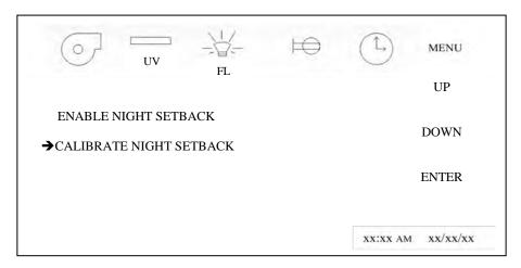
Step 3: At this point, the night setback is active and the butterfly valve will begin to close. Now measure the inflow volume using a Direct Reading Instrument of inflow velocity measurement method. The goal is to reduce the inflow volume to the following values, which represents approximately 100 fpm (.51m/s) inflow, or may be set at any other values within the damper operational range of 30% to 80%.
