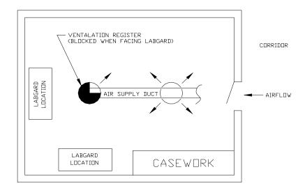
If drafts or other disruptive air currents exceed the inflow velocity of the cabinet through the access opening, the *potential* exists for contaminated air to exit or enter the work zone area of the cabinet. It depends on the severity of the air current. **REMEMBER: A BIOSAFETY CABINET IS NO SUBSTITUTE FOR GOOD LABORATORY TECHNIQUE.**
