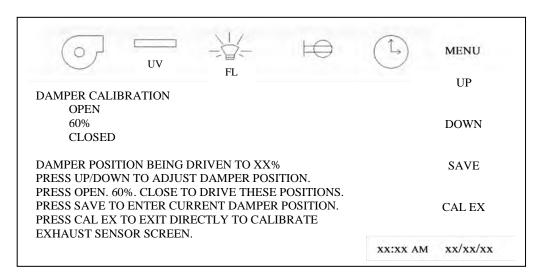
Set damper position to 60° on the display. NuAire recommends using the damper position at 60° to minimize static loss and maximum controllability of the system. However, THE DAMPER CAN RANGE FROM 35° TO 75° FOR ITS NOMINAL SETPOINT. ANY POSITION OUTSIDE THIS RANGE WILL SEVERELY LIMIT THE CONTROL SYSTEMS ABILITY TO ACCURATELY CONTROL THE EXHAUST VOLUME.
