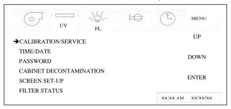
Entry into the Calibration/Service functions requires a service password for entry. After pressing the Calibration/Service menu item, a password screen will appear. The default password is "9876". Once the service password is entered, the Calibration/Service menu will appear.
