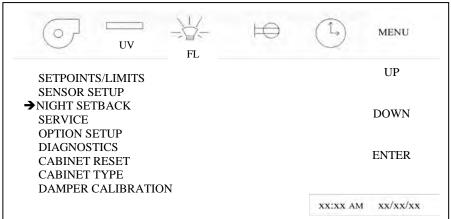
Step 1: Determine how night setback is initiated. If using contacts on main control board, proceed to step 2. If using the display icon, enable night setback option by performing the following:
