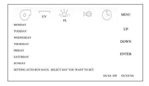
Once into the selected day, press UP or DOWN to enter the on/off times. Use the >> and << to select hours or minutes. Press SWITCH to toggle between auto time on and auto time off. Press SAVE after each time entry. Press DIS to disable auto timer for the day being reviewed. Repeat auto timer function for each day as desired.
