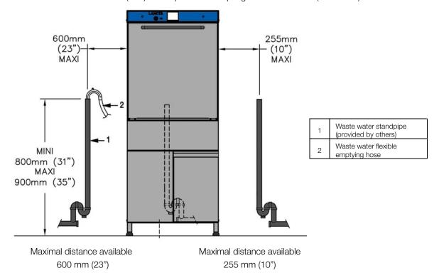
THE DISCHARGE TUBE MUST BE LOACATED IN THIS AREA.
