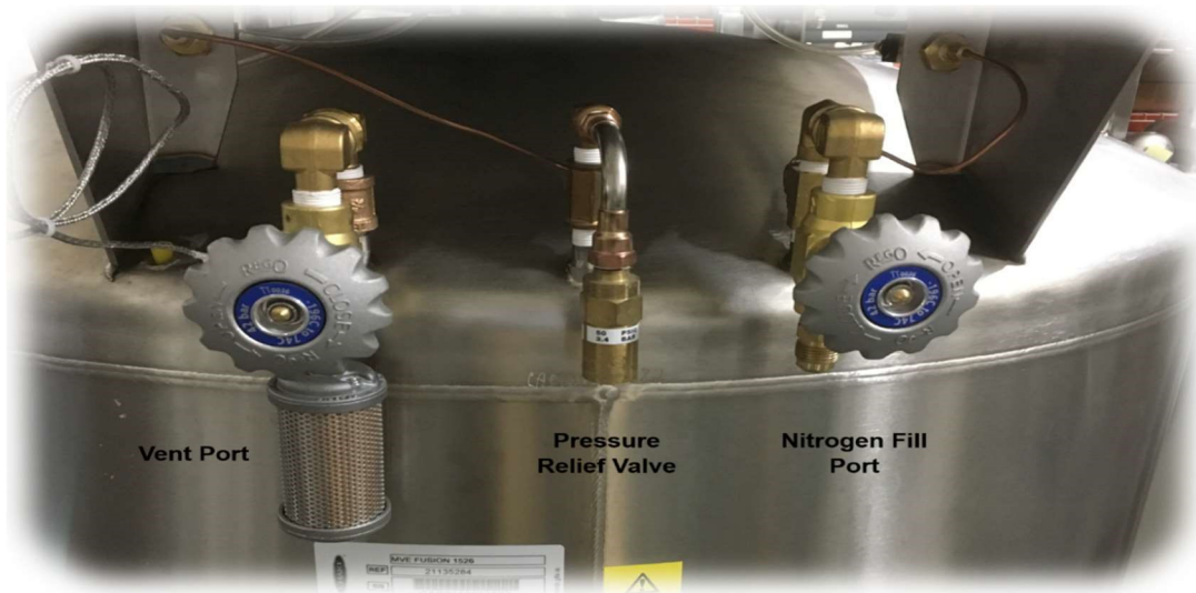
Figure 5: Left to Right: Vent (Overfill) Valve, Relief Valve, and Fill Valve
