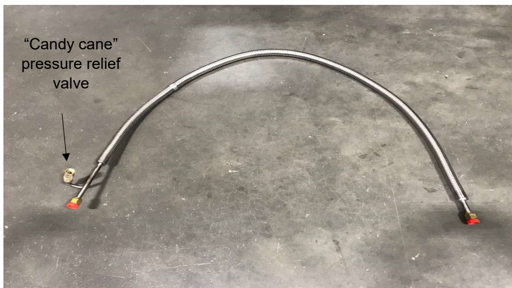
Figure 7: Transfer hose with the candy cane relief valve included
