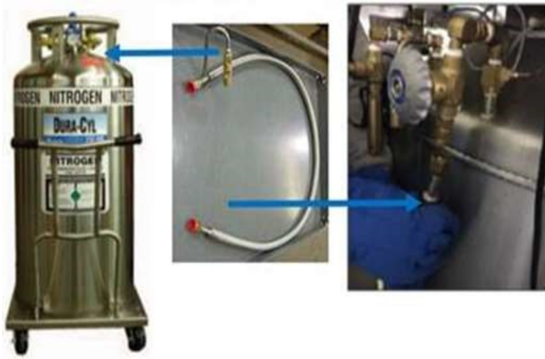
Figure 15: Connecting Supply Tank to the MVE FUSION
