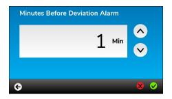
**Minutes Before Deviation Alarm:** The default setting of 1 means that the chamber temperature must deviate for more than 1 minute before the alarm activates.
