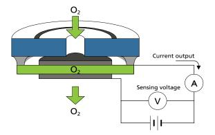
The  $O_2$  molecules diffuse through the Zirconia layer in the sensor, causing a voltage build-up. The voltage then creates an electrical current flow which is detected by the sensing circuit in the incubator.
