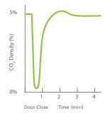
The infrared CO<sub>2</sub> control system is designed to establish, maintain and recover CO<sub>2</sub> concentration to the desired setpoint. This sensor provides accurate control and accuracy with fast recovery to setpoint following door openings. The PID control algorithm eliminates overshoot as CO<sub>2</sub> is restored, typically in less than 2 minutes.
