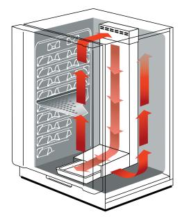
Active Background SafeCell UV The primary components of this technique are found in copper enriched stainless steel interior protection and destruction of airborne contaminants by UV light exposure within the positive airflow plenum. Both work continuously to inhibit the growth of organisms on interior surfaces of walls and shelves, and by destroying the DNA of pathogens that enter the chamber through door openings or normal handling.
