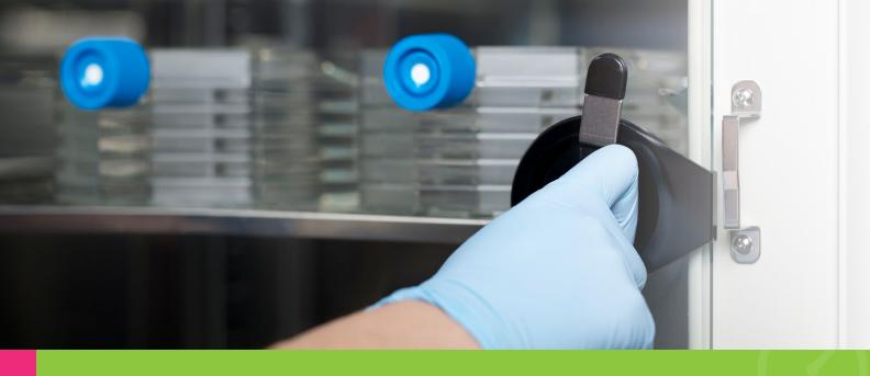
PHCbi brand cell culture incubators are available in a selection of CO<sub>2</sub> and multigas CO<sub>2</sub>/O<sub>2</sub> models. Gas blends are managed by a microprocessor controller which calculates gas percentages based on input from CO<sub>2</sub> or O<sub>2</sub> sensors. Gas setpoints and actual levels are displayed on the main control panel for easy reference.
