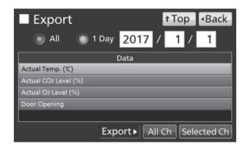
\* When both of the Auto-lock function and the User-ID mode are ON (refer to page 76~79), inputted User-IDs for unlocking the outer door are also exported.
