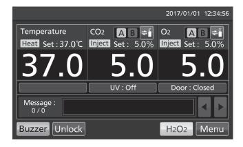
2. CO<sub>2</sub> gas supply line A is changed to B.
