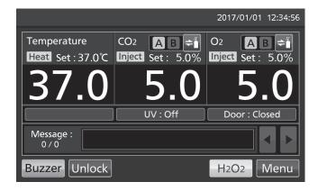
· In the User-ID mode, when pressing Unlock key on the Top screen, User-ID input box is displayed. Input the User-ID and its release password of Auto-Lock.
