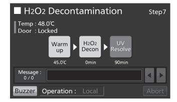
**15.** When the  $H_2O_2$  decontamination is completed, the  $H_2O_2$  Decontamination Step8 screen is displayed.
