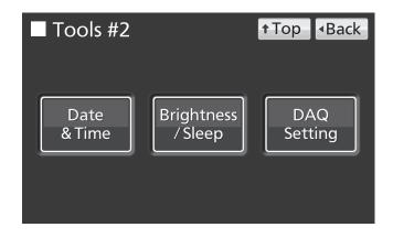
**4.** On the Brightness/Sleep screen, each setting of brightness and sleep is available. Press Apply key to save the input value and setup. The display returns to the Tools #2 screen.
