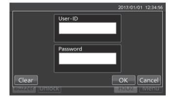
$\cdot$  When the inputted User-ID or its password is incorrect, Notice dialog box is displayed. Press OK key, and then input the correct User-ID or its password.
