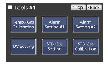
**4.** On the Alarm Setting #1 screen, input each parameter. Press Apply key to save the input value. The display returns to the Tools #1 screen.
