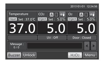
2. N<sub>2</sub>/O<sub>2</sub> gas supply line A is changed to B.
