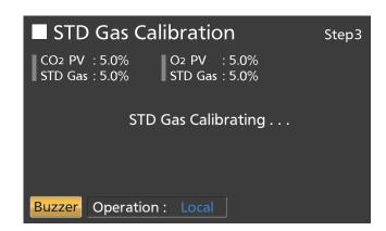
**10.** After completion of gas density calibration, display leads the STD Gas Calibration Step5 screen.  $O_2/CO_2$  incubator returns to the normal operation.
