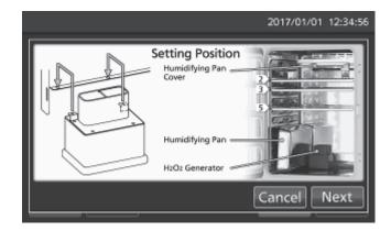
**13.** On the  $H_2O_2$  Decontamination Step1 screen, the system check starts automatically. If the system is normal, the display leads the  $H_2O_2$  Decontamination Step2 screen. When the system is abnormal, refer to Table 10 on page 94.
