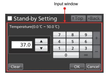
Note: While the input window is open, it is not possible to operate Top key and Back key.
