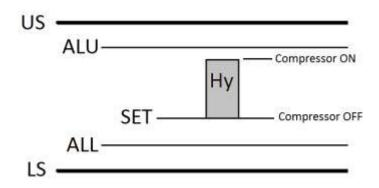
During the normal operation, the refrigerator's (or freezer's) compressor would turn on and off, in order to maintain the cold temperature in the storage chamber.
