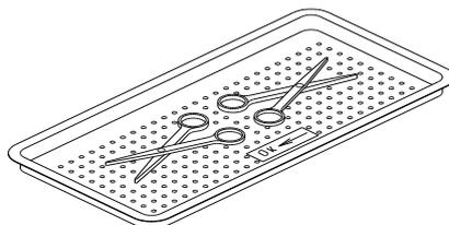
13. Disassemble or sufficiently loosen multiple-part instruments prior to packaging to permit the sterilizing agent to come into contact with all parts of the instrument.
