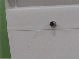
Thermocouple through Access Port & Access Port Plug
