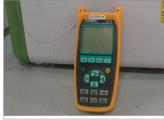
NIST Traceable Temperature Measuring Device
