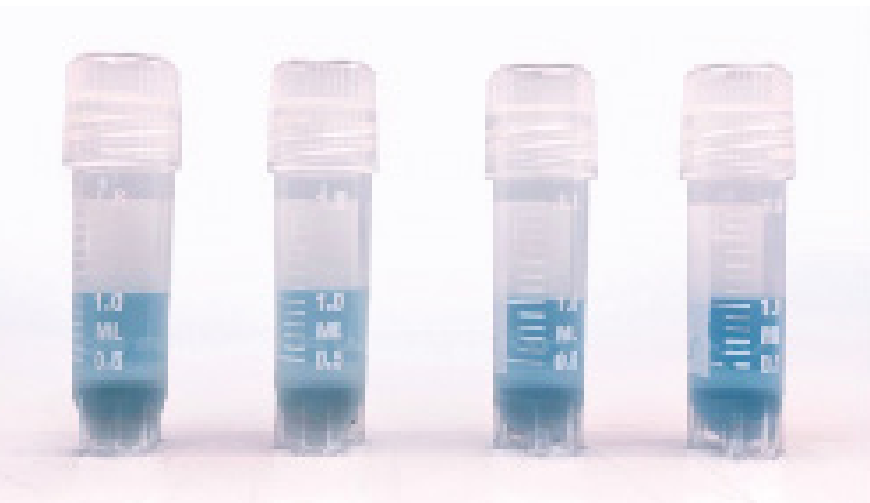
Fig. 1 - Ice Nucleation layer (in dark blue) formed after controlled nucleation in 2 mL vials.
