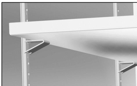
1. Install the shelf clips in the slots of the shelf standard mounting rails located on the sides of the chamber interior, 4 clips per shelf.
