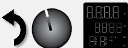
Turn the Over Temperature Limit dial counterclockwise until the temperature controller display goes dark.
