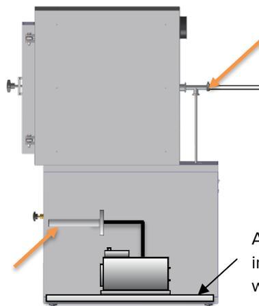
1. Connect a vacuum supply to the KF-25 vacuum port on the back of the oven.
