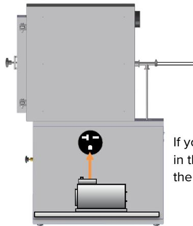
If you have installed a vacuum pump in the cabinet, you may plug it into the NEMA 6-20R power outlet.
