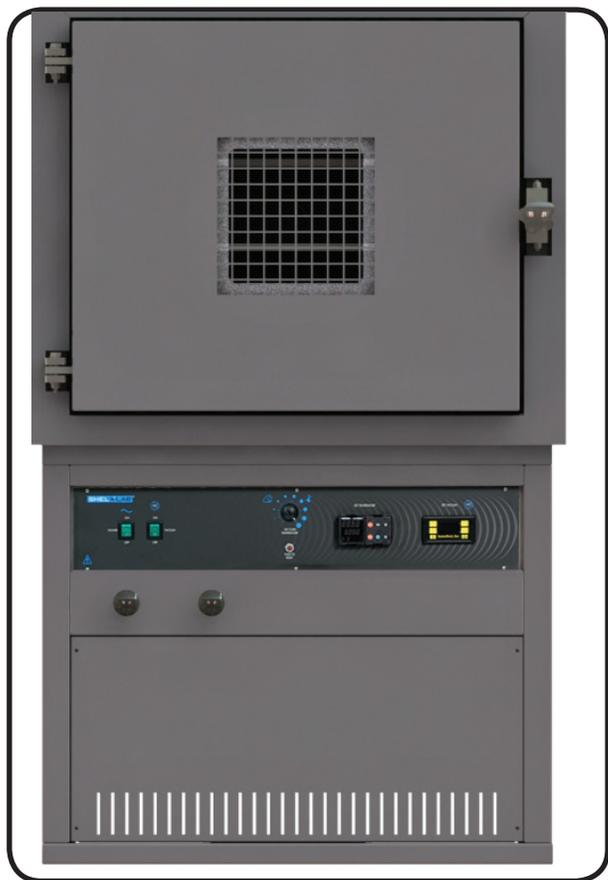
The SHEL LAB Model SVAC9-2 includes a Watlow temperature controller that can be programmed to perform multiple ramp and soak profiles. A digital vacuum gauge shows chamber vacuum level in measurements of Torr and m/Torr. The display range is 760 Torr down to 0 mil Torr. A secondary independent high limit controller provides overtemperature safety protection.
