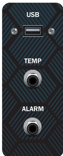
**TEMP Port:** 4 – 20mA analog output describing the current chamber temperature.
