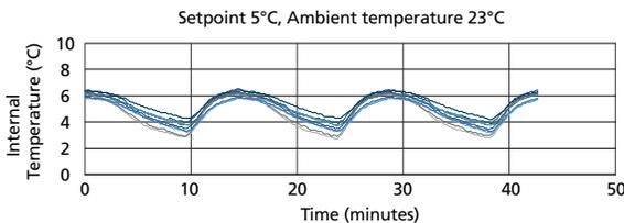
As interior air temperature stabilizes at the desired setpoint, large mass storage volume sustains tight temperature uniformity of the load inside the insulated cabinet.
