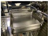
4. Place the complete humidifying pan cover with part number 624 230 4555 over the humidifying tray and make sure to place it against the back wall of the incubator.
