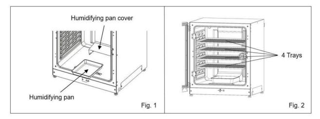
3. Place the smaller humidifying pan with part number 624 230 4548 on the bottom of the incubator and make sure to place it with the long side against the back wall of the incubator so water accumulated on the dew stick will drip in this humidifying pan.
