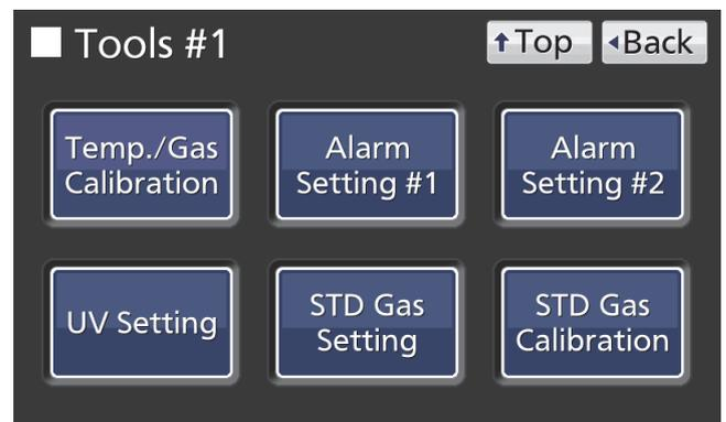
4. On the UV Setting screen, each setting of UV is available. Press Apply key to save the input value and setup. The display returns to the Tools #1 screen.
