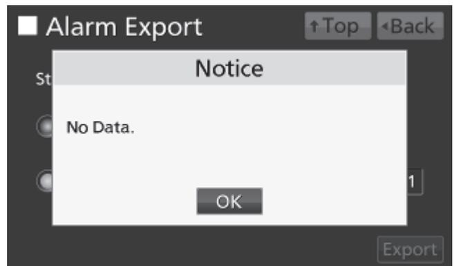
7. Even after completion the export of alarm log data, Information dialog box is displayed. Press OK key.
