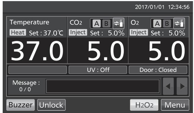
2. CO<sub>2</sub> gas supply line A is changed to B.
