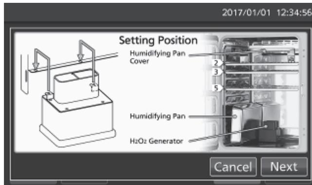
13. On the H<sub>2</sub>O<sub>2</sub> Decontamination Step1 screen, the system check starts automatically. If the system is normal, the display leads the H<sub>2</sub>O<sub>2</sub> Decontamination Step2 screen. When the system is abnormal, refer to Table 10 on page 94.
