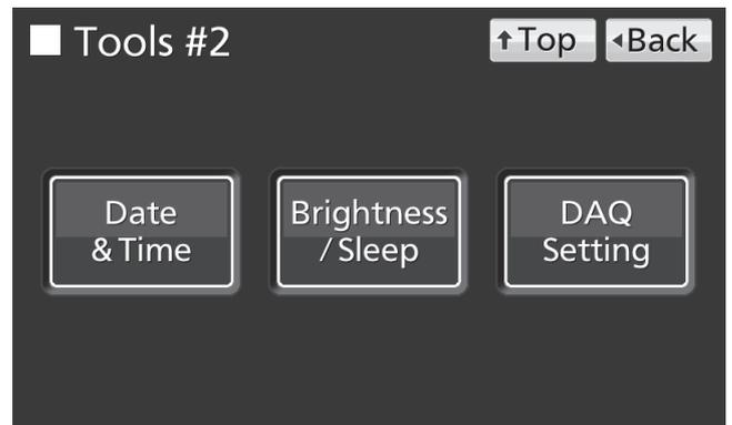
4. On the Brightness/Sleep screen, each setting of brightness and sleep is available. Press Apply key to save the input value and setup. The display returns to the Tools #2 screen.
