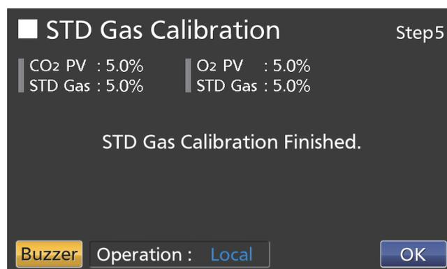
11. On the STD Gas Calibration Step5 screen, press OK key to return to the Tools #1 screen. On the Tools #1 screen, press Top key to return to the Top screen.
