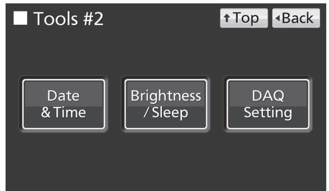
4. On the Date & Time screen, input the present date and time. Press Apply key to save the input value. The display returns to the Tools #2 screen.
