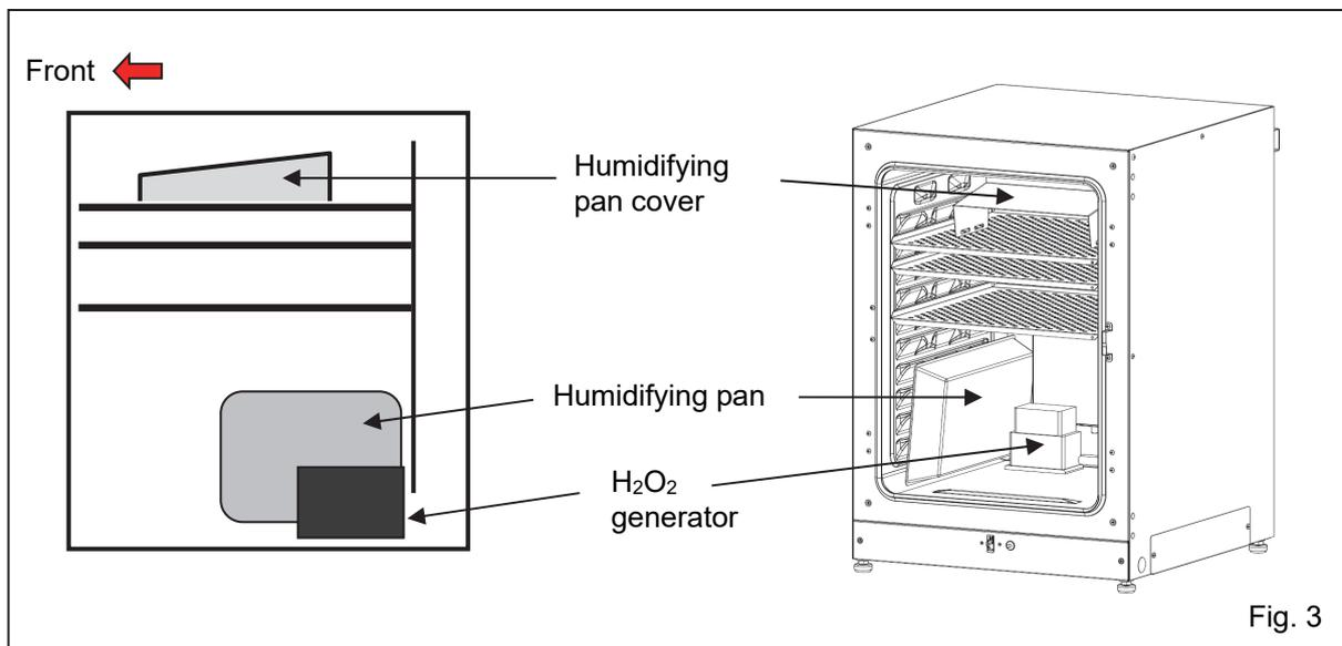
10. Make sure that the duct, the fan and the H<sub>2</sub>O<sub>2</sub> generator are securely attached (refer to Fig. 1 to 3 on page 97). After that, close the gastight split doors, the inner door and the outer door.
