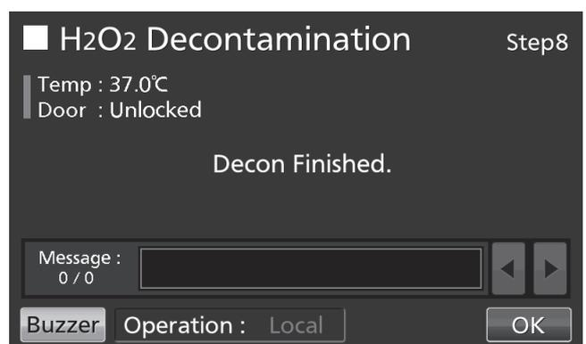
17. Dilute the remaining H<sub>2</sub>O<sub>2</sub> reagent in the H<sub>2</sub>O<sub>2</sub> generator with a large volume of water and dispose of it. Rinse and wash the H<sub>2</sub>O<sub>2</sub> generator with distilled water. Then keep the H<sub>2</sub>O<sub>2</sub> generator in a clean environment outside of the chamber.
