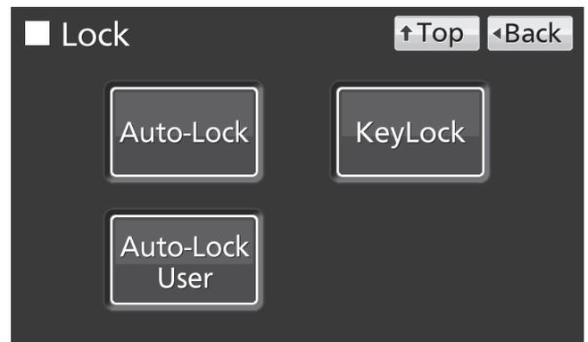
4. On the Auto-Lock screen, by holding the Auto-lock slide key and sliding it left, the Auto-lock is turned to OFF. Press Apply key to change Auto-lock OFF, and the display returns to the Lock screen.
