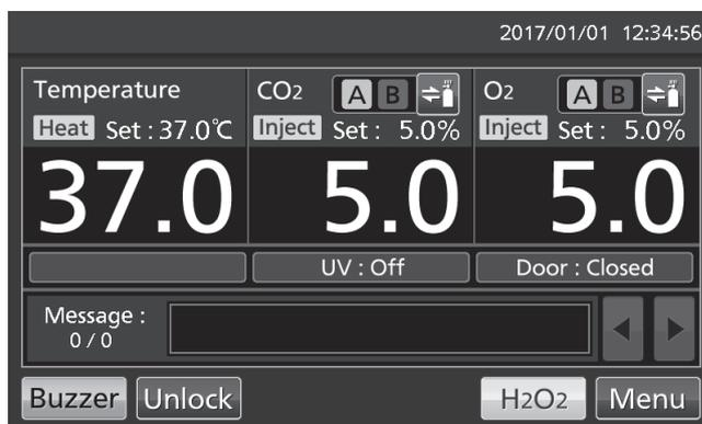
12. Finally make sure that the inner attachments and the H<sub>2</sub>O<sub>2</sub> generator are attached correctly. After confirmation, press Next key to lead the H<sub>2</sub>O<sub>2</sub> Decontamination screen.
