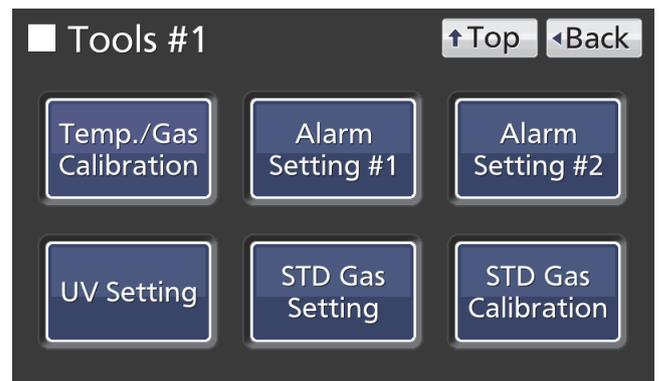
7. On the UV Setting screen, by holding the UV 24h Mode slide key and sliding it right, the UV 24h Mode is turned to ON. Press Apply key to start the UV 24-hour mode. The display returns to the Tools #1 screen.
