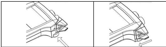
The electrode clip is an electrode holder that can be placed next to the display on either side of the housing.
