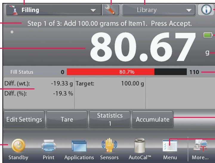
Battery life indicator when powered by optional battery pack (for High Capacity models only)
