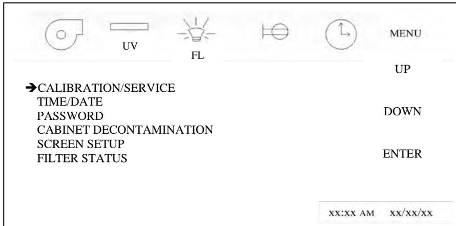
Entry into the Calibration/Service functions requires a service password for entry. After pressing Calibration/Service menu item, a password screen will appear. The default password is "9876". Once the service password is entered the Calibration/Service menu will appear.
