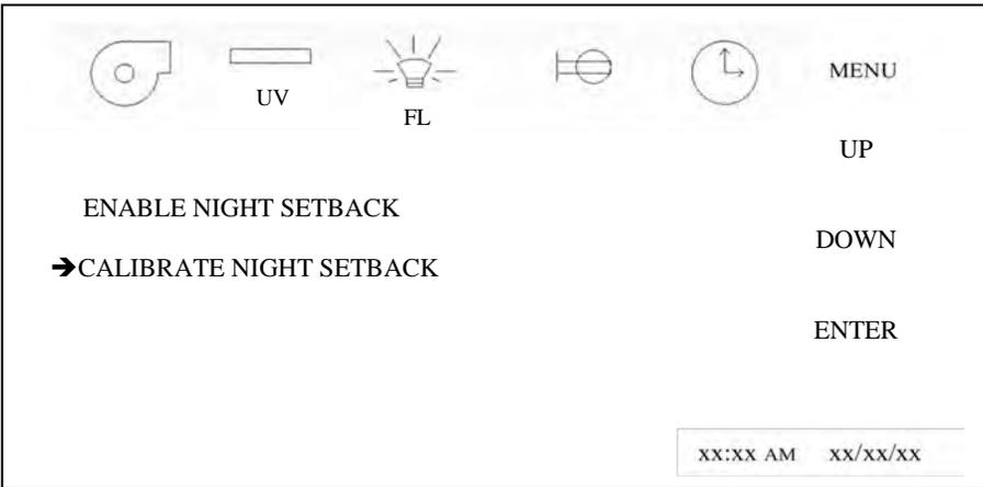
Step 3: At this point, the night setback is active and the butterfly valve will begin to close. Now measure the inflow volume using a Direct Reading Instrument of inflow velocity measurement method. The goal is to reduce the inflow volume to the following values, which represents approximately 100 fpm (.51m/s) inflow, or may be set at any other values within the damper operational range of 30% to 80%.
