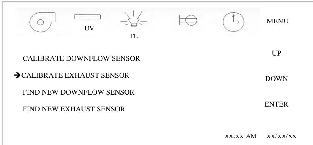
Press CALIBRATE EXHAUST SENSOR to access individual sensor calibration screen.
