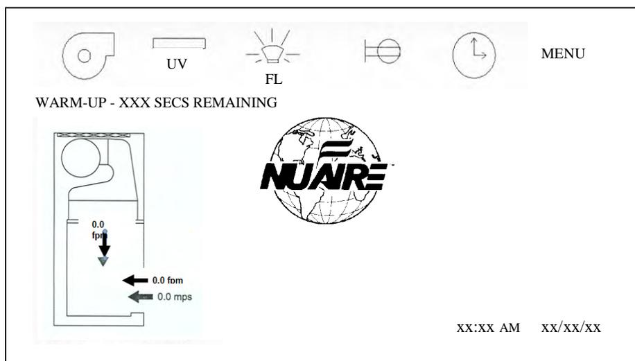
Once the warm-up period is complete, airflow readings and all system functions will operate and be displayed.
