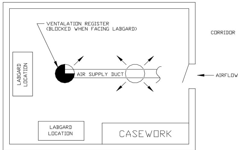
If drafts or other disruptive air currents exceed the inflow velocity of the cabinet through the access opening, the *potential* exists for contaminated air to exit or enter the work zone area of the cabinet. It depends on the severity of the air current. **REMEMBER: A BIOSAFETY CABINET IS NO SUBSTITUTE FOR GOOD LABORATORY TECHNIQUE.**
