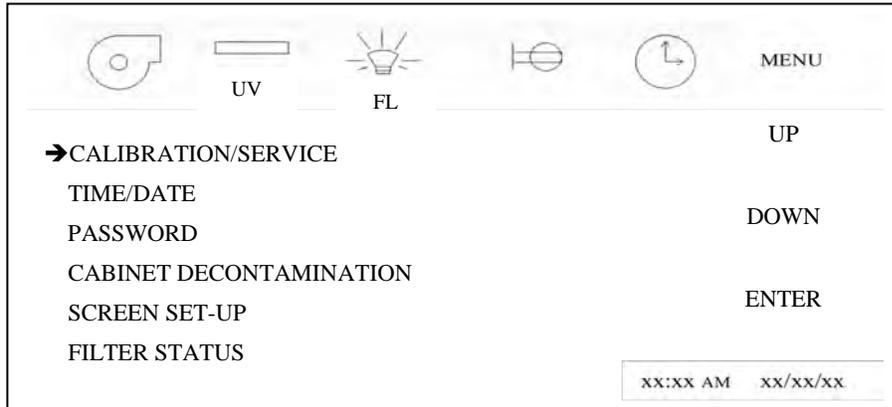
Entry into the Calibration/Service functions requires a service password for entry. After pressing the Calibration/Service menu item, a password screen will appear. The default password is "9876". Once the service password is entered, the Calibration/Service menu will appear.
