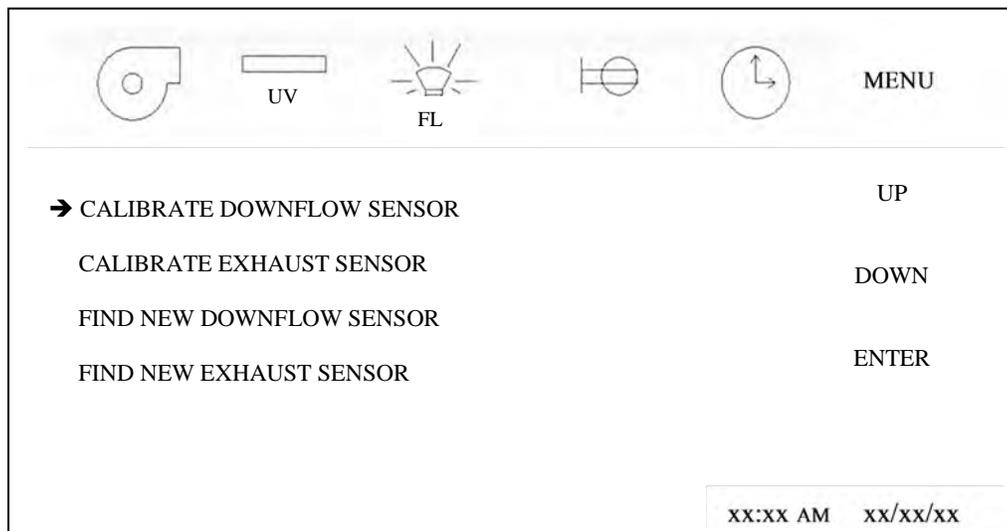
Step 2: Press CALIBRATE DOWNFLOW SENSOR to access individual calibration screen. Press BLOWER switch to on. Allow blower to run for one minute or until downflow readings are steady.
