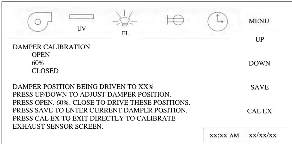
Set damper position to 60° on the display. NuAire recommends using the damper position at 60° to minimize static loss and maximum controllability of the system. However, **THE DAMPER CAN RANGE FROM 35° TO 75° FOR ITS NOMINAL SETPOINT. ANY POSITION OUTSIDE THIS RANGE WILL SEVERELY LIMIT THE CONTROL SYSTEMS ABILITY TO ACCURATELY CONTROL THE EXHAUST VOLUME.**
