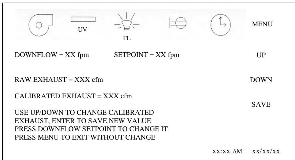
Step 2: Turn on motor/blower and spot check a few downflow points to verify downflow is close to the desired setpoint of 60 fpm  $\pm$  5 fpm.
