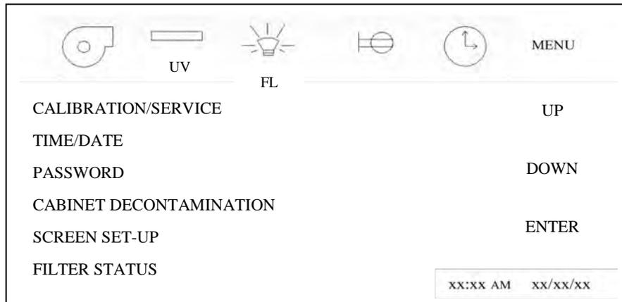
Entry into the Calibration/Service functions requires a service password for entry. After pressing the Calibration/Service menu item, a password screen will appear. The default password is "9876". Once the service password is entered, the Calibration/Service menu will appear.
