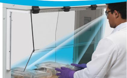
**A slanted polycarbonate sash** provides unrestricted view of the work zone while reducing glare
