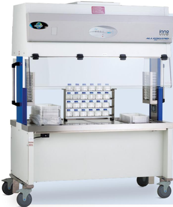
The AllerGard NU-620M is designed specifically to accommodate Innovive<sup>®</sup> disposable mouse cages while employing similar airflow mechanics as our other dual-sided models, by flushing the work zone with a vertical “piston of air” to preserve aseptic conditions.
