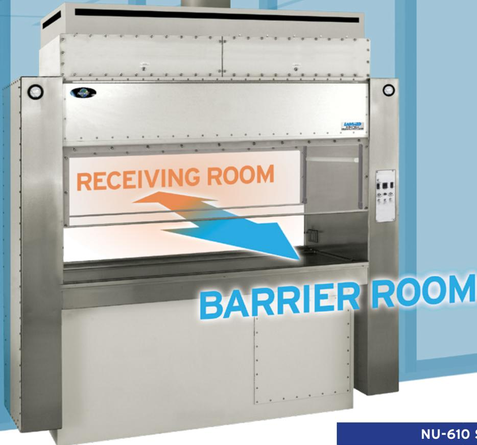
The LabGard® ES (Energy Saver) NU-610 Class II, Type A2 Dual Access Laminar Airflow Biosafety Cabinet is built directly into the wall of your laboratory, which makes it easy to transfer new animals into a facility or move them between different rooms. NuAire builds each NU-610 model to fit your lab's specific needs. The NU-610 uses a Minihelic™ pressure gauge to constantly monitor and display airflow
