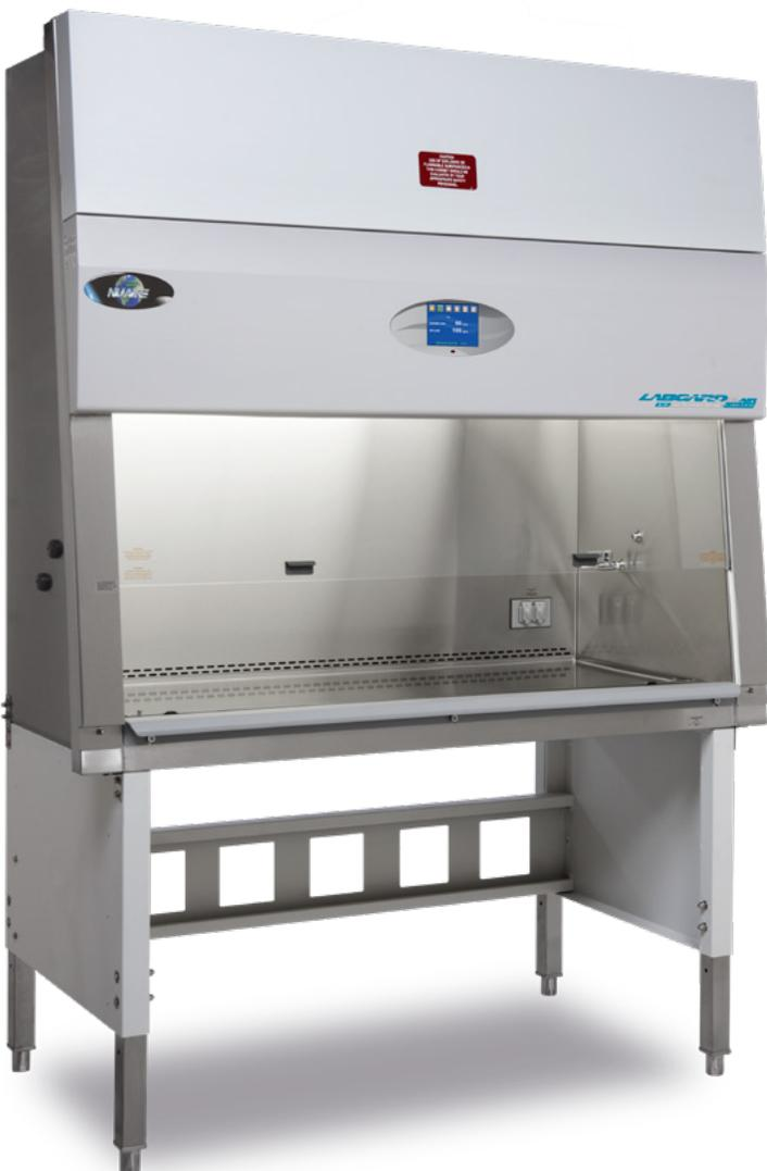
The LabGard® ES (Energy Saver) AIR Limited Model NU-545 Class II, Type A2 Biosafety Cabinet is a bench/table top model with available base stand options. The Energy Saver DC ECM motor is controlled to airflow set points via the TouchLink™ central control system. The touch-screen control system utilizes two dual digital thermistor airflow sensors that provide automatic compensation for both filter loading and line voltage variances to maintain constant air volume control.
