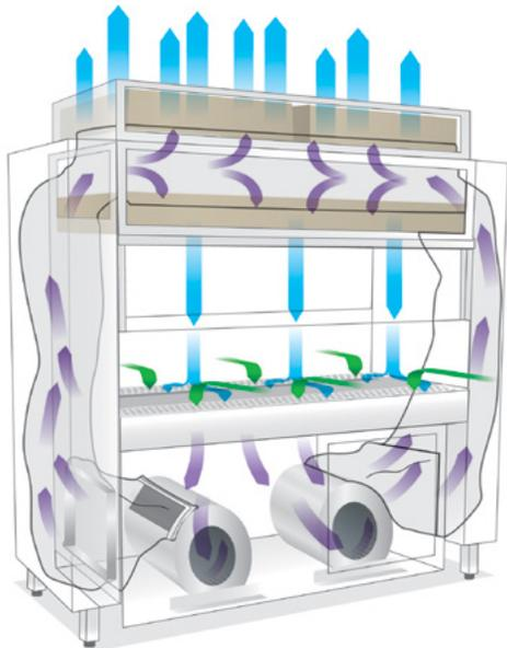
All sizing and feature options are fully customizable to fit your lab's specific needs. The NU-610 is typically built as a Class II Type A2, which normally exhausts back into the room, but this unit is fully capable of connecting directly into your facility's HVAC network. The pass-through system can also be optimized with any NuAire ergonomic options and accessories to ensure your personnel's continued comfort.
