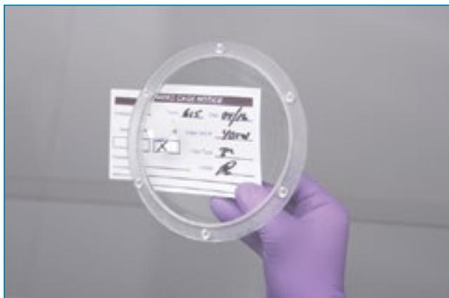
A magnifying glass is installed in the window sash to enhance text written on animal identification cage cards.
