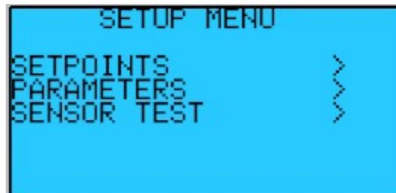
This screen allows access to the listed set up screens. Press the
