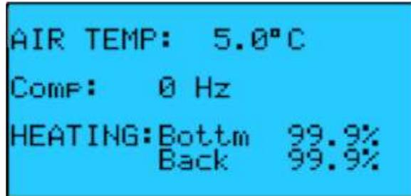
This screen shows the control probe reading, the resultant variable frequency which drives the compressor and hence the refrigeration, the percentage output of the electric heaters and the status of humidity control (humidification/dehumidification).
