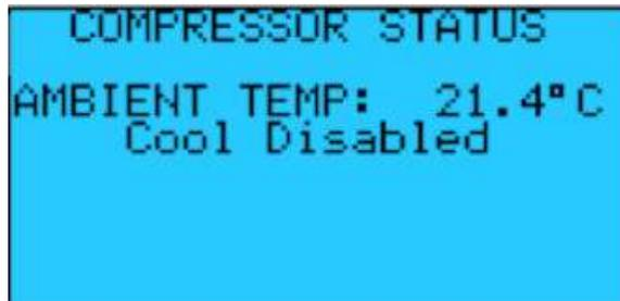
This screen shows the ambient probe reading and the status of both the main and auxiliary refrigeration systems
