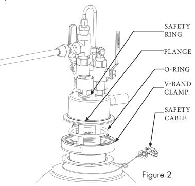
of the hose. If liquid nitrogen is trapped between the valves of the liquid cylinder and the LWD, it has no escape path as it warms and expands. The resulting pressure can cause the hose to rupture and may cause personal injury. The current model LWD is equipped with a pressure relief valve. Previous versions of the LWD must be used with a transfer hose equipped with a pressure relief valve.
