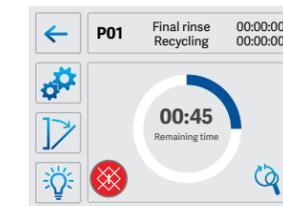
**Cycle in Process.** A real-time status screen displays time remaining until cycle completion and links to cycle detail screens with the touch of a button.
