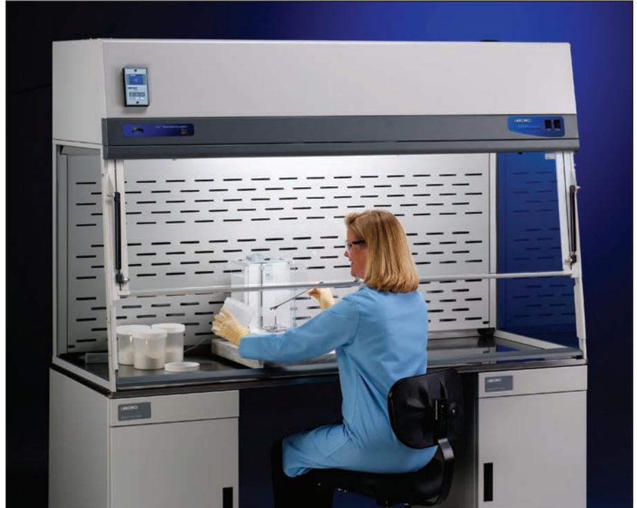
*Since the XPert Filtered Balance System includes a built-in blower and HEPA filter mounted in the upper plenum, no outside ducting is required.*
