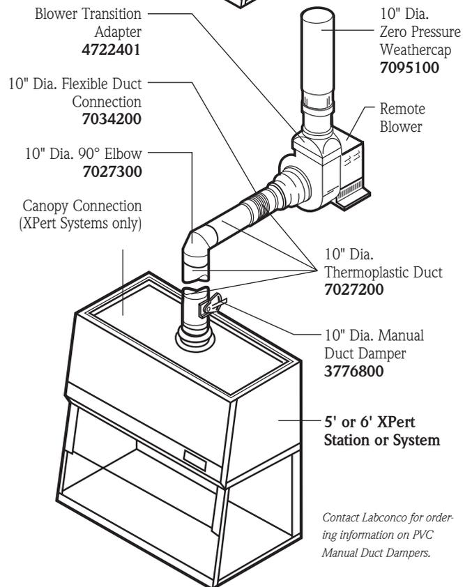
Contact Labconco for ducting options for XPert Enclosures connected to Remote Blower 7068200, 7068300, 7068400 or 7068500. See inside back cover for Typical Exhaust System for 8' XPert Enclosures.
