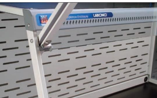
sash opening to the baffle in a single pass. The lower section provides more airflow at the bottom to help minimize the potential for air to roll forward toward the sash opening.
