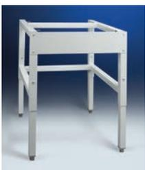
Support XPert TXE Equipment Enclosures. Powder-coated 1.75" tubular steel. Adjustable to eight height positions at installation in 1" increments from 27.5" to 34.5". Available with fixed feet or 5" diameter casters. Shipping weight 100 lbs. (45 kg)
