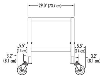
\* Telescoping Base Stands do not isolate vibration. When using sensitive balances in the enclosure, a marble slab may be necessary to reduce vibration from outside influences.
