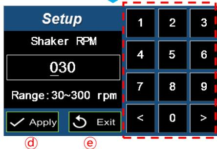
① TOUCH the RMP Shaker value, the screen turns to the Shaker setting screen
