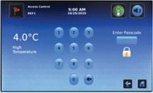
**Integrated Electromagnetic Access Control** - Offers secure access to the refrigerator via the i.C3® Information Center (i.Series®) or Horizon Access Control Keypad (Horizon Series™).
