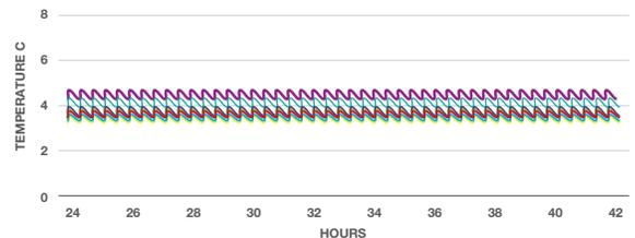
**Recovery** - Faster recovery after prolonged door openings. Forced-air circulation keeps contents at the right temperature even when the unit is opened multiple times per hour for stocking, inventory counts and product retrieval.
