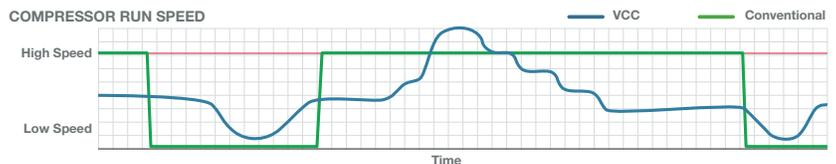
The OptiCool™ cooling system uses intelligent sensors to monitor operating conditions. When the door of the unit is opened, the VCC runs at a higher speed to deliver optimal temperature performance. When the temperature stabilizes, the VCC runs at a lower speed, resulting in lower energy consumption.
