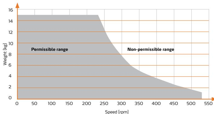
The displayed values were determined with flat weight blocks and without further superstructures on the shaking platform and are only used for orientation. The actual maximum possible speed must be determined and defined by the user in an appropriate manner, depending on the process in each individual case. It is not possible to give a general manufacturer recommendation for the different scenarios due to the application-specific parameters.
