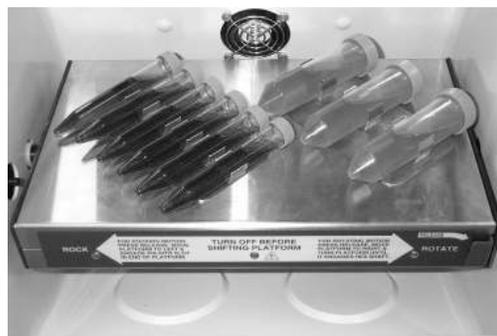
**NOTE:** When rotating tubes, rotate the magnetic platform by hand before starting, to check the clearance of the tubes to the chamber walls.
