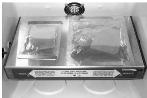
Various size tubes can be placed on the magnetic platform in different orientations to produce different motions within the tubes. First select the size clip plate required. The large clips hold 28-30mm dia. (50ml) tubes, the medium clips hold 15-17mm dia. (15ml) tubes and the small clips hold 10-13mm dia. (1.5-2.0ml) tubes. One clip plate of each size is supplied. The platform can hold up to eight plates (see Accessories). Push the tubes into the clips.
