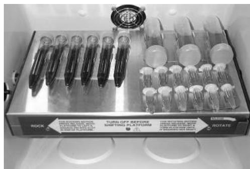
Positioning the plates as shown below will produce a rolling or rocking motion in the tubes.
