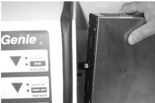
Now hold up the right side of the platform, while depressing the blue lock release. Screw the lock shaft into the hole in the magnetic platform making sure the blue lock release is depressed. When the lock shaft is screwed all the way in, let go of the lock release.
