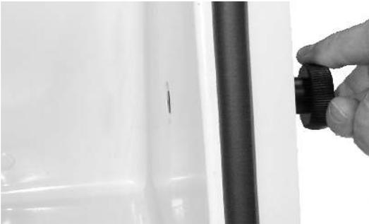
Grab the magnetic platform with the label side up, so that you can read the label. Hold the platform in the chamber and insert the hex shaft on the left side of the chamber into the hex hole in the magnetic platform. You may need to rotate the platform slightly to align the shaft with the hole.
