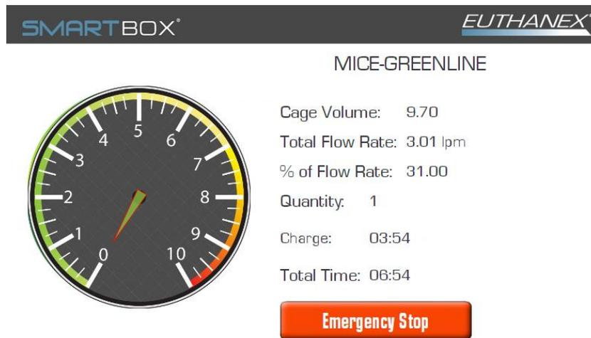
**Stage 2 Dwell:** Gas flow stops and the cages remains fully charged with CO<sub>2</sub>.
