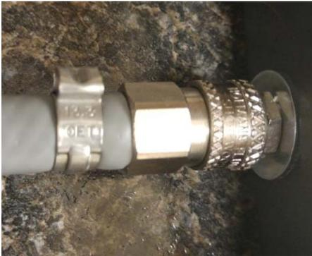
3. Connect the supplied cage hose from the output of the Prodigy (located on the right side) to the input valve on the Euthanex Lid. The unit will support operation of 3 cages in a cycle.
