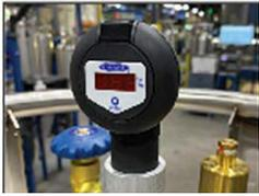
The C-Stic Liquid Level Gauge offers improved accuracy and reads zero to 100% full.
