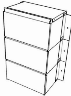
Empty Battery Box
