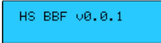
Initial screen: Displays software version temporarily during initialization. After initialization, Press
