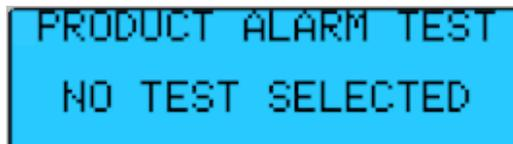
Press the ENT key to move the cursor to the NO TEST SELECTED data field. Use the Up or Down Arrow key to scroll through the tests. When the correct test is displayed press the ENT key to start the test. Press the ESC key to return to the System Status screen.
