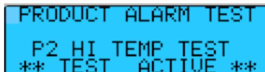
This screen will be displayed when a test is active. To end a test, press the ENT key to move the cursor to the TEST data field and use the Up or Down Arrow key to scroll through the tests until “NO TEST SELECTED” is displayed. Press the ENT key to end the test.
