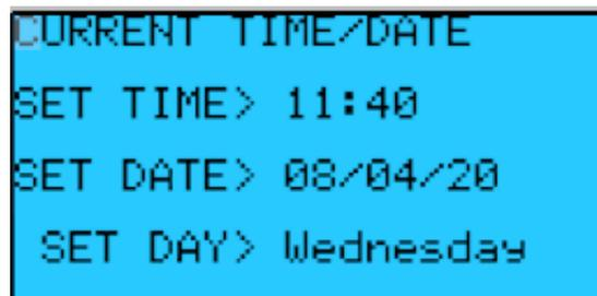
Note: This setting allows the user to edit the real-time clock. The system will reference the real-time clock for scheduling and alarm logging purposes.
