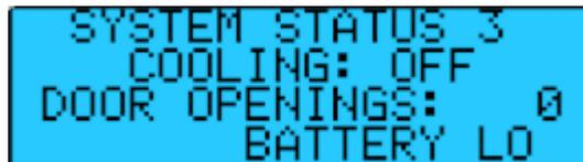
This screen displays the status of the refrigeration system, the number of door openings and the status of the backup battery.
