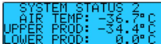
This screen displays the product temperature probe and the reading from the control probe
