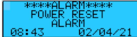
The ALARM HISTORY screen will display the last alarm that has occurred. The controller will store the last 100 alarms that have occurred. To view the Alarm History Log, press the ENT button to move the cursor to the alarm #. Using the UP and Down Arrow buttons scroll through the stored alarms.
