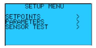
To access the setpoints, parameters, and senor test sub-menus, press the enter key to move the cursor, then press up or down key to enter the desired sub-menu.
