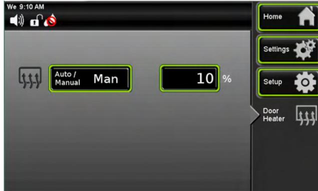
In Manual mode, the door heater is a fixed output value regardless of temperature set point. This setting should only be used in units that have active cooling with temperature set points well above the low-end range.
