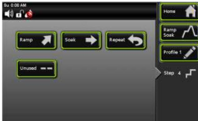
Choose the Unused
