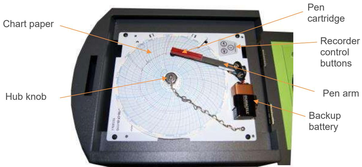
Press and hold the “change chart” button on the recorder (#3) for approximately one second until the pen begins to move to the left of the chart and then release the button. Wait until the pen has completely moved off of the chart. To remove the chart paper, unscrew (counter-clockwise) the chart “hub” knob at the center of the chart. Remove the old chart paper and position the new one so that the correct line coincides with the time line groove on the chart plate.
