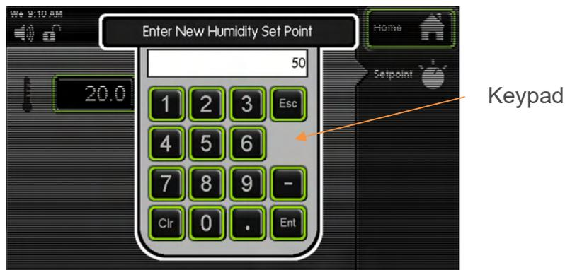
Enter the new humidity setpoint on the keypad as desired and press
