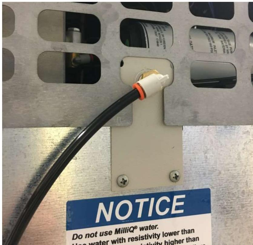
A water inlet fitting on the back of the unit and ¼" black tubing are provided to connect the water supply to the chamber. Connect an appropriate water supply to the fitting. Incoming line pressure should be regulated to not exceed 80 psi.
