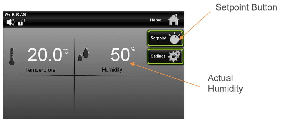
To set the humidity setpoint, press the
