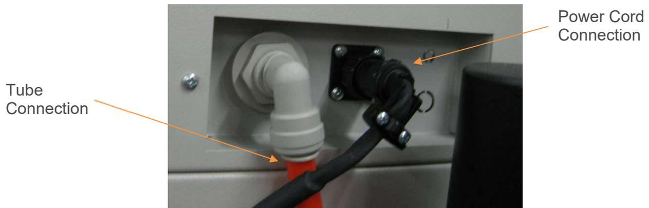
3. Attach 3/8" orange tubing from the chamber to the flow meter outlet.
