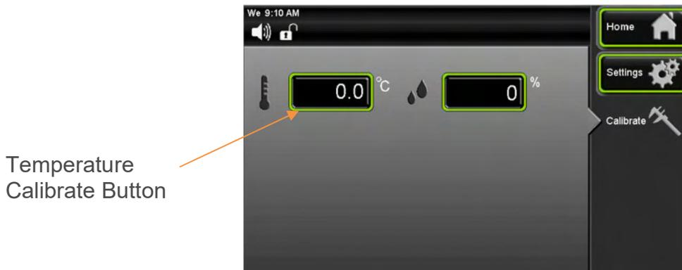
At the calibrate screen, press the
