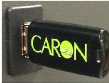
The DLOG301 option provides the customer with a means of logging data electronically for viewing at a later date. Logged variables are Temperature, Humidity, CO<sub>2</sub> and Light Intensity (but only if the chamber is equipped with those features.) All data is time-stamped with year, month, day of the month, hour, minute, 24 hour time (ISO 8601 format). This data is stored internally in the chamber in non-volatile memory.
