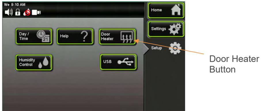
From the Setup screen press the
