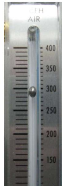
4. Adjust the flow meter adjustment knob so the flow is 300 SCFH.
