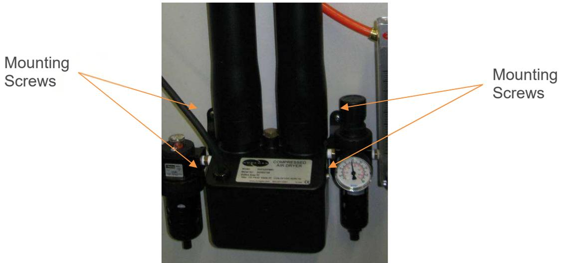
2. Connect dryer package power cord and 3/8" orange tubing into the dryer panel on the chamber
