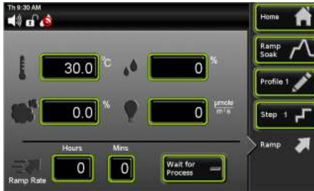
Ramp rate allows a user to control the rate which parameters (temperature, humidity, CO<sub>2</sub>, lights) change when transitioning to a new setpoint. This allows for a more gradual change than otherwise would occur.
