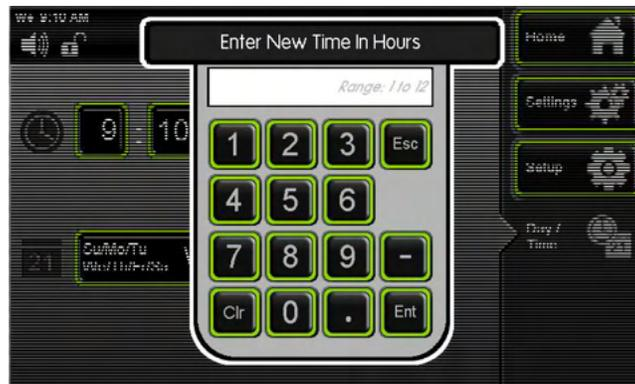
The Enter New Time in Hours window will appear. Enter the hour by using the keypad and pressing
