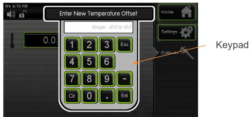
Enter the temperature offset by using the keypad and pressing
