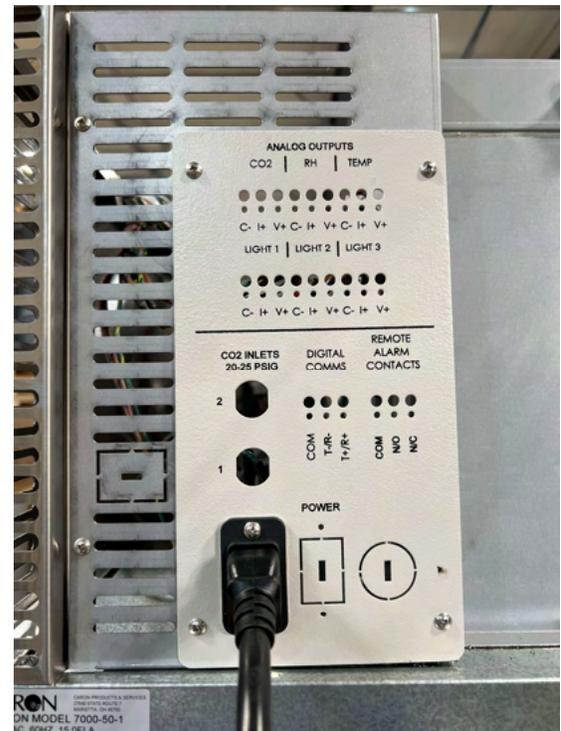
Analog outputs provide either a milliamp (4-20mA) or voltage (0-5V) signal output to represent each of the displayed temperature (and humidity) values. These options can be used for connection to in-house data acquisition, recorder, or alarm system. The temperature parameter (only) is adjustable in its scaling and is accessible at the Analog Output screen.
