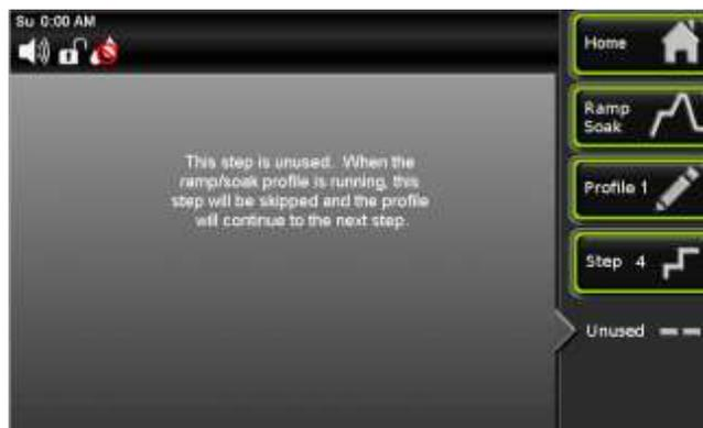
So when the Ramp, Soak or Repeat condition is not chosen for a step, the ramp profile program will skip over those unused steps.
