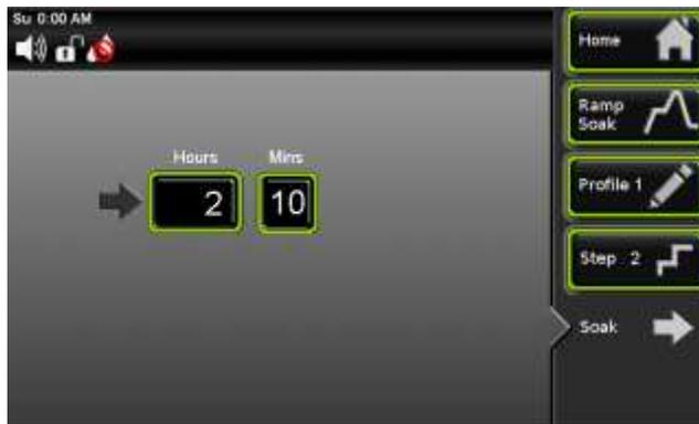
When finished entering values, press the
