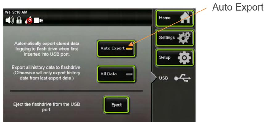
Select the 'Auto Export' feature on the USB menu screen. Insert the flash drive into the chamber's USB port. A new .csv file is automatically created on the flash drive with all the stored history data. The file name nomenclature is "DATE END YYYY-MM-DDTHH-MM\_ .csv".
