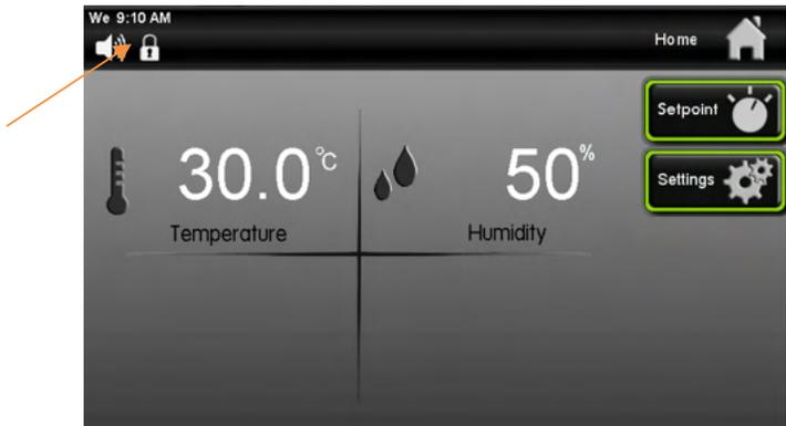
When any button is pressed on the home screen the following pop-up window will appear. If the
