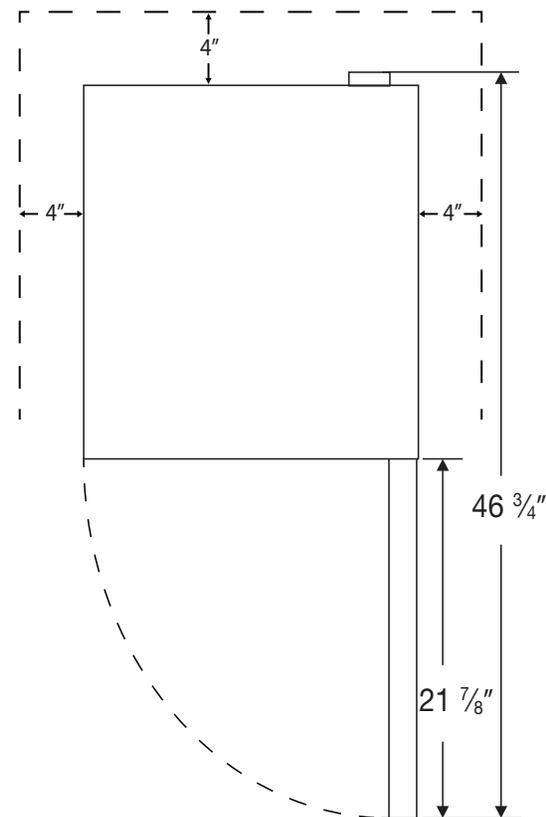
**NOTE: Ventilation Requirements – Minimum 4" clearance on sides and back**
